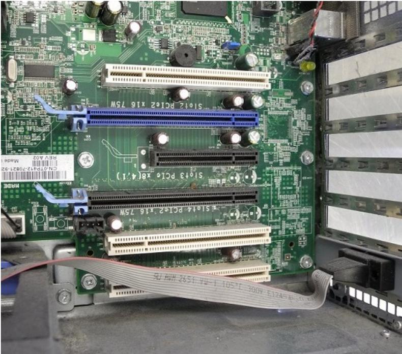
5. Insert the SafeNet Luna PCIe HSM card into the connector. It should go straight in – angling the card might cause it to bend. The card is properly seated when no portion of the gold-colored contacts of the card-edge protrudes above the connector socket.
