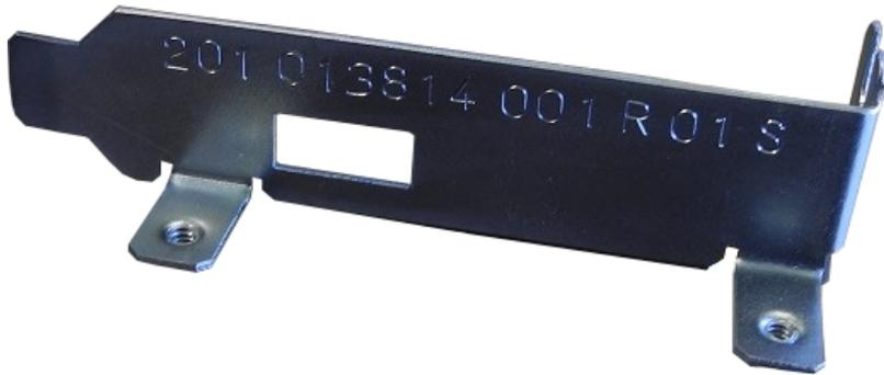
4. Align the SafeNet Luna PCIe HSM card with the vacant, unpowered slot. You might need to introduce the tip of the card-hold-down bracket first (the silver-metal part along the back edge of the card), in order to properly align the card with the connector.
